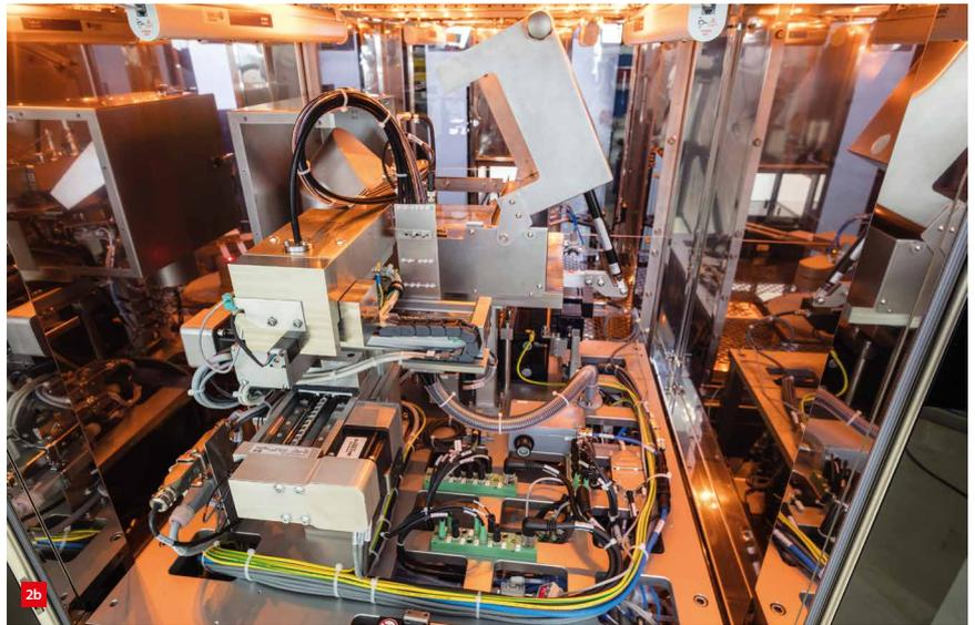
Another important design requirement was the operation of the cleaning wiper tape and the cassette from which it is dispensed. For moving the tape smoothly, in both directions, the effects of wetting and friction had to be taken into account. An innovative clamping mechanism featuring two spline axes was also designed, for rapid manual exchange of the tape cassettes.
